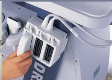
Cart supports three selectable transducers (Two active)
